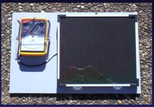
A solar cell transforms light energy into electrical energy. Each cell is composed from two layers of silicon with upper and lower electrodes.
